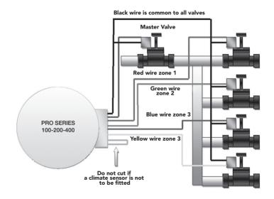
Do not connect the 9V battery until you have connected the various zone cables.
